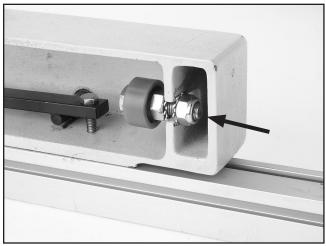
Figure 28. Rip fence height adjustment.
